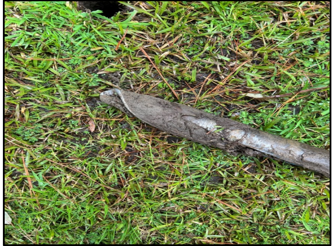
Figure 15. BH1 sample profile consisted of grey brown light clay and wet soil.
